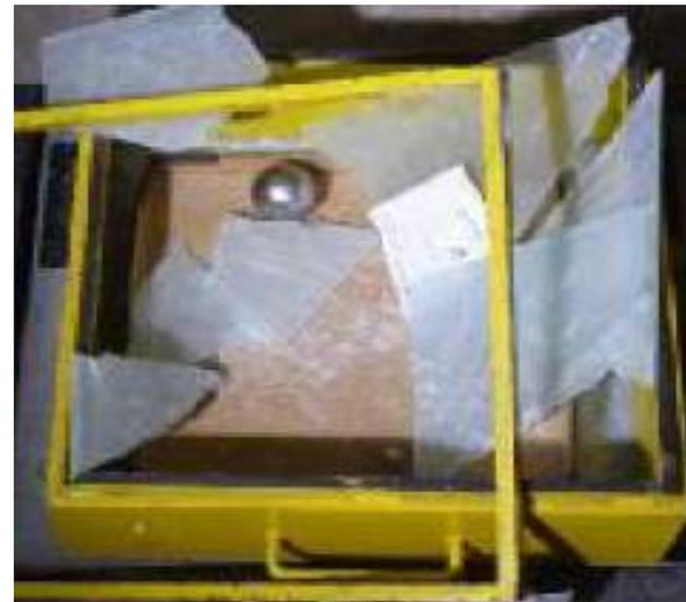
There are several international standards in the glass industry to evaluate the safety performance of laminated safety glass and corresponding interlayers. In this one pager results are discussed from the ball drop testing according to the DIN 52338 standard on laminated safety glasses made with different types of interlayers. (Pictures: Left: Test passed, Right: Test failed)
